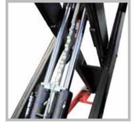
• Sicurezza meccanica • Mechanical locking system AT-ATLT
