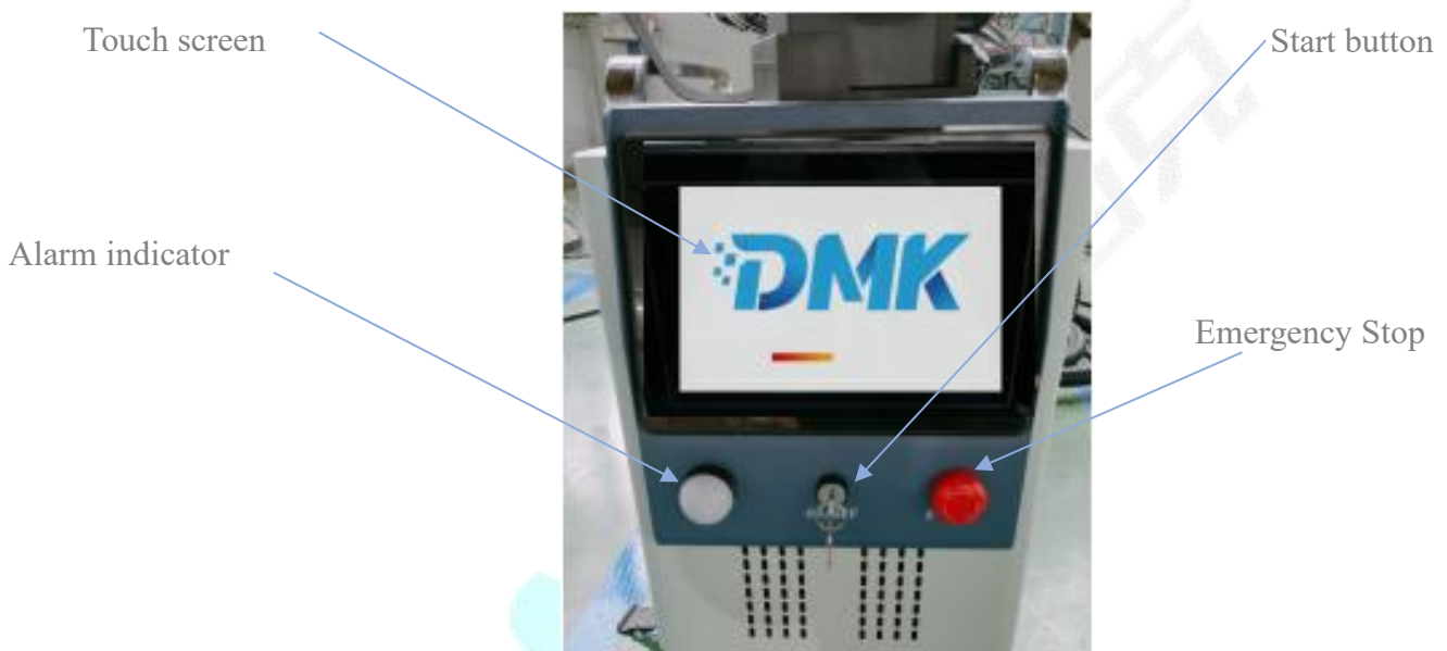
Fig3.3 Front operation panel of DPL-300W
