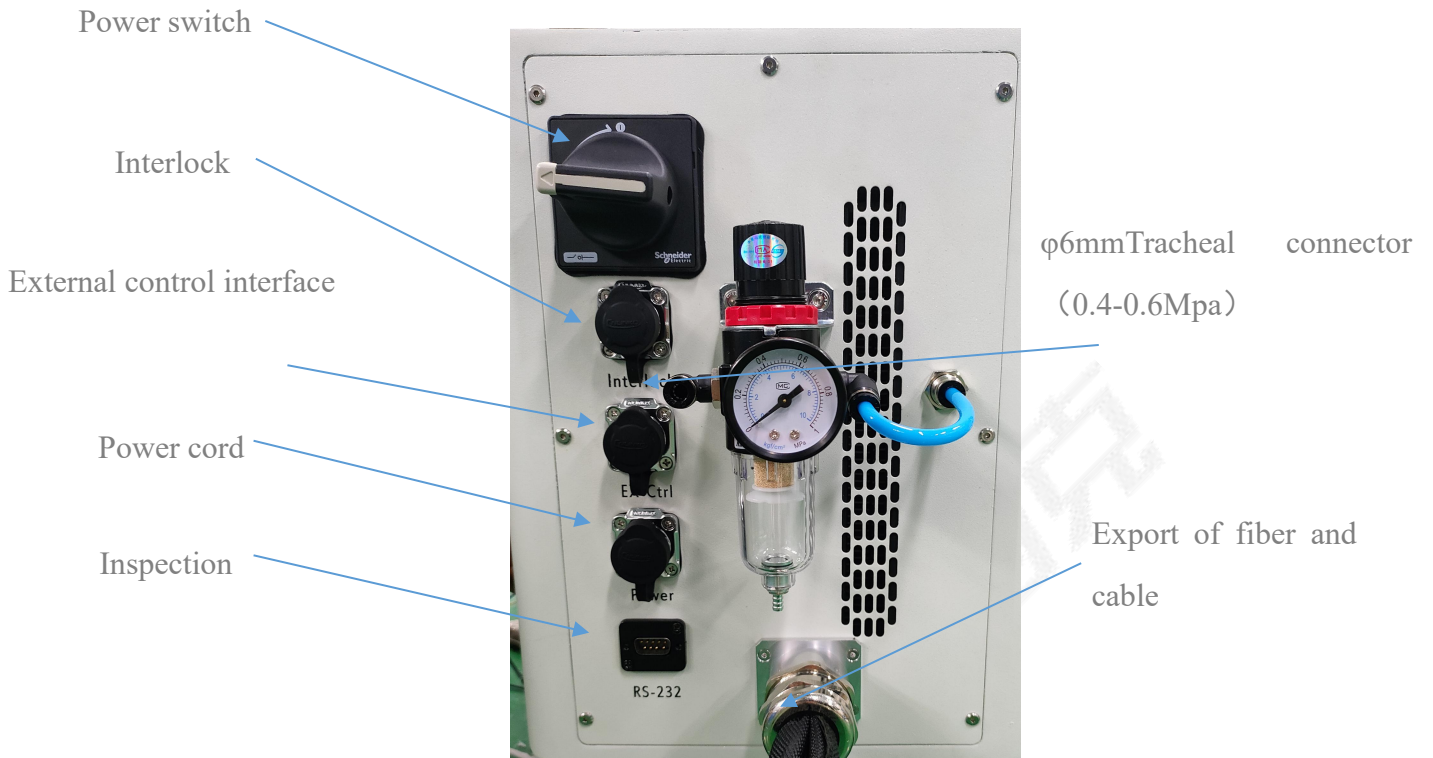
Fig3.4 Rear operation panel of DPL-300W
