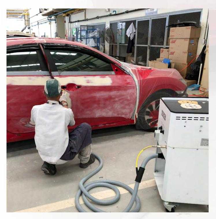
The self-cleaning filter system, unique in its range of reference, is derived from the centralized industrial systems and allows to keep the filters always clean which do not require any maintenance. The use of a tool automatically starts the suction turbine that will turn off when you stop working, thus reducing fuel consumption.
