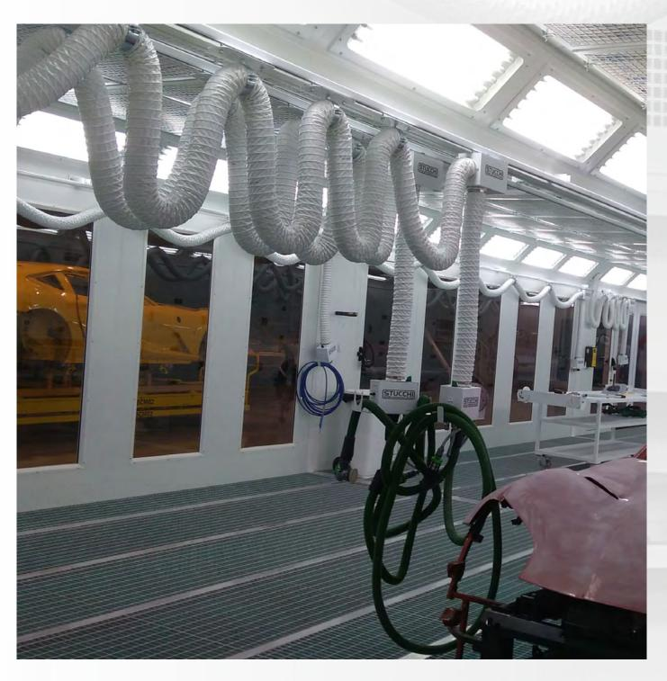
It enables users to position the service control unit next to the workstation and avoid therefore installing bulky loose cables or routing pipes across the work areas. It's ideal to have more security at the workplace and to have a more professional and tidier organisation.
