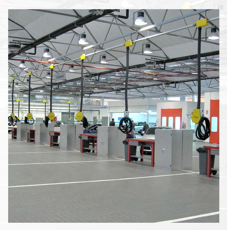
Start-up is automatic with both electrical and pneumatic tools. The suction system can be started using the remote start selector present on the hexagon.
