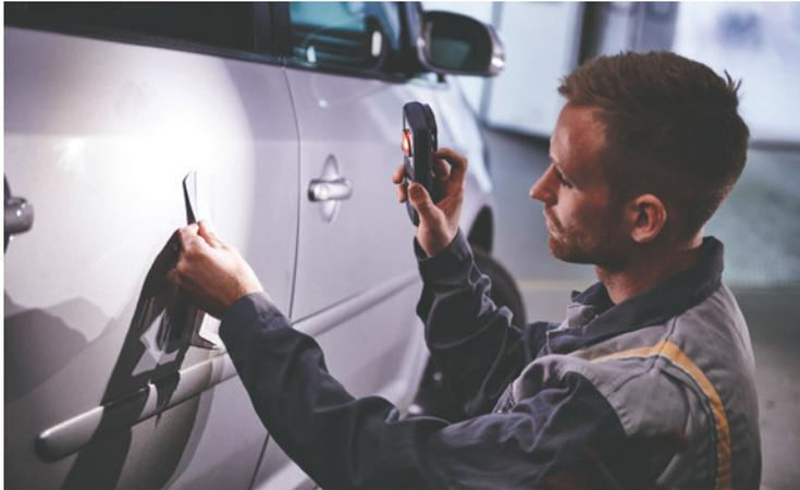
The Sunmatch color matching light reduces the chance of costly paint mistakes due to poor color matching. The Sunmatch, with its ultra-high CRI of 95 at 4500 Kelvin does an amazing job of replicating sunlight, giving you the best color match results.
